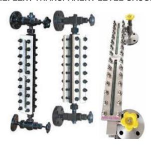
NRG offers a series of level indicators. Designed to measures the level of liquid in reactor tanks. The reflex level gauge is used for the measurement of liquid level for high pressure or high temperature or toxic liquid storage tanks. The reflex level gauge has a single prism glass mounted on one side of the chamber and uses the basic optical principles of light reflection to upgrade the expression of the liquid level in the process tank.
